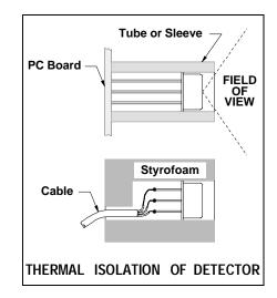
First, the instrument or device using the detector should have a completely closed housing - with plastic or laminated metal
