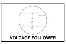
Detectors with a **voltage follower** offer a low output impedance and a high signalto-noise ratio. The units are composed of a sensing element, an ELTEC thick-film high megohm load resistor and a field
