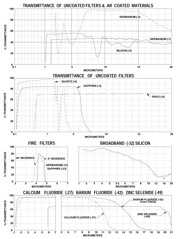
this filter does not have an anti-reflection coating and thus has transmission around 50%. Also see the -32 filter.
