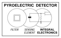
Thus to produce a more practical lowimpedance voltage signal, electronics are packaged within most pyroelectric detectors. Naturally, the impedance conversion can be accomplished outside the detector, but most users choose integral electronics for reasons of convenience, reliability, shielding and cost.
