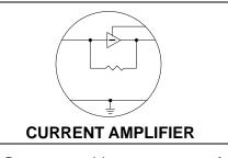
Detectors with a **current mode amplifier** have very high voltage responsivity. In fact, the signal strength is often great enough to eliminate the need for further amplification. However, in applications with low level inputs or demanding signal-to-noise requirements, the current amplifier should not be chosen.
