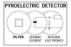
The filter protects the crystal and internal electronics from physical damage and air drafts. The filter, when properly selected, will block wavelengths of no interest and pass those desired.
