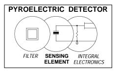
gives a substantial margin of protection because a thin wafer can heat up fast in response to an intense pulse of incident radiation.
