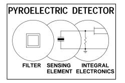
A detector consists of a **filter**, a **sensing element**, and **integral electronics**. The filter restricts incoming radiation to a wavelength band of interest, the crystal responds to the incident energy and produces a signal, and the integral electronics assist in mating the signal with other equipment. ELTEC makes available a variety of filters, crystals, and electronics so as to best meet the needs of specific applications. ELTEC detectors are also available without electronics.
