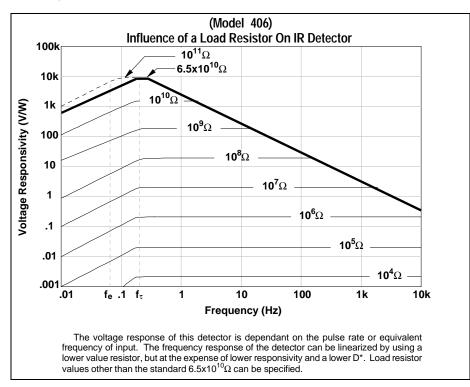
effect transistor. The thermal time constant of the crystal establishes the potential low frequency response. This thermal limit in conjunction with the effective capacitance of the sensing element (including stray) and the high megohm load resistor determine the detector's frequency response. As the sample curve shows, responsivity decreases as load resistors are chosen to extend flat response.
