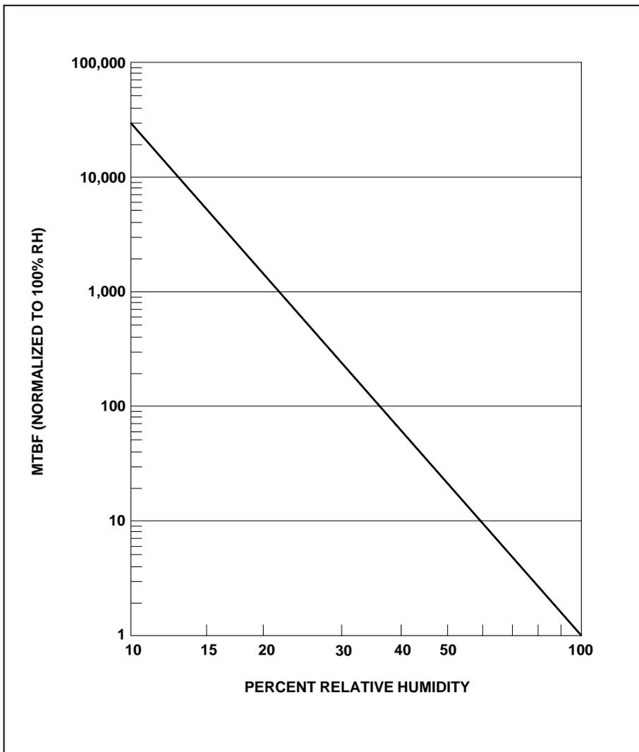
Figure 12. Corrosion failure rate versus relative humidity (at constant temperature).
