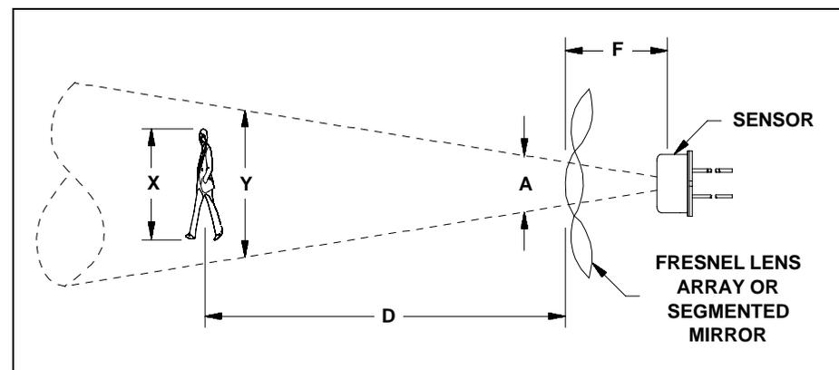
Figure 6. Signal strength optical dependency.
