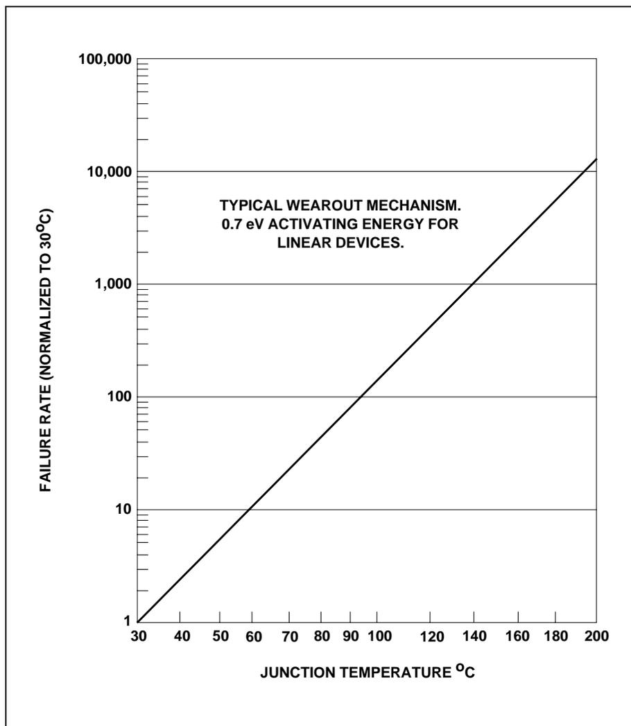
Figure 11. Failure rate as a function of junction temperature.
