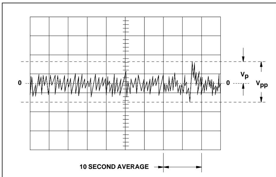
Figure 8. Peak-to-peak noise determination.
