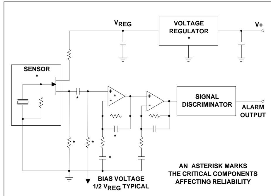
Figure 5. Typical intruder alarm circuit.
