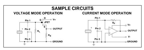
$<sup>^{1}</sup>$ Integrating mode load resistor R<sub>L</sub> 5 x 10 $^{6}$   $\Omega$ .
